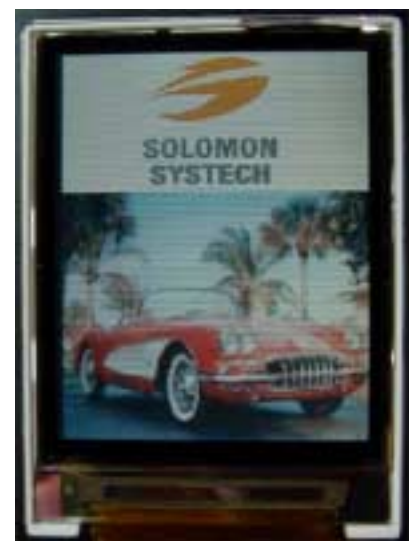
Figure 1 - 1.9" QCIF+ module using Solomon Systech's TFT driver SSD1278.
