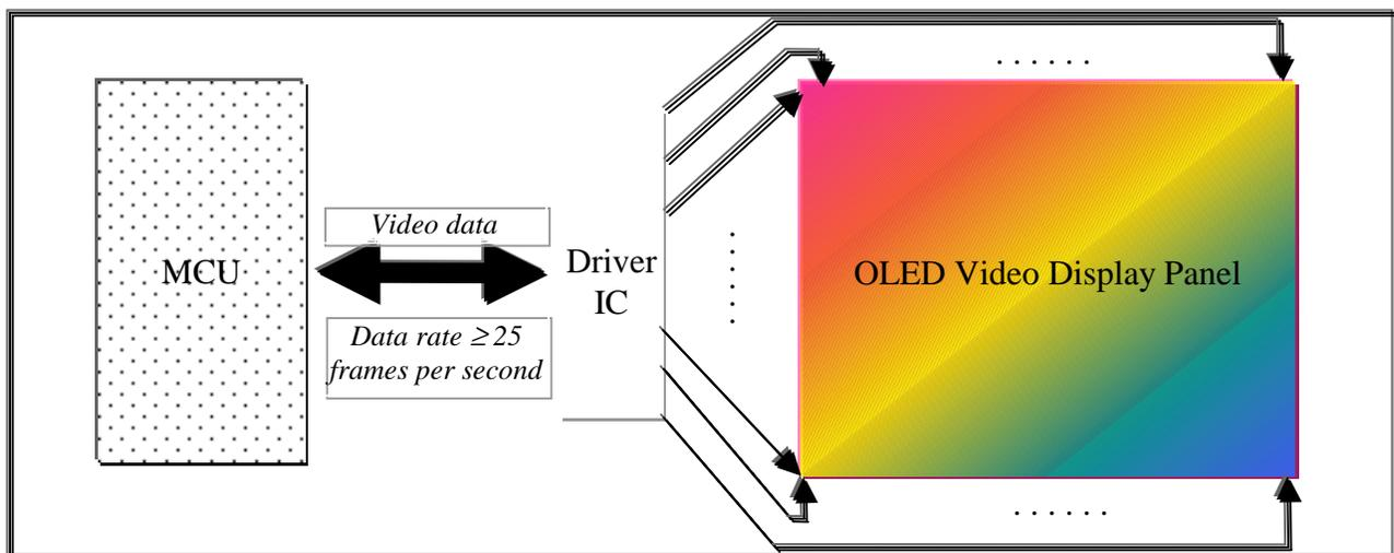
The SSD1339 is a single-chip driver IC with controller for the OLED panel. It supports panel resolution up to 132RGBx132. The driver reveals realistic image colors by providing 262K true color. To achieve such high color resolution, the MCU communication data width has been increased to 18-bit, ensuring both fast and smooth video display performance.
