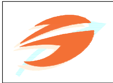
Ghosting effect without over-drive scheme on slow response LCD
